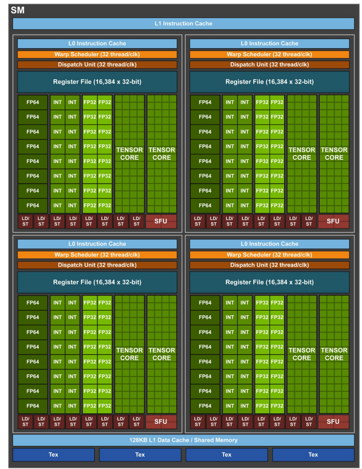
Examples: Google Cloud TPU, Nvidia GPU Architectural Scalability With Tiling
